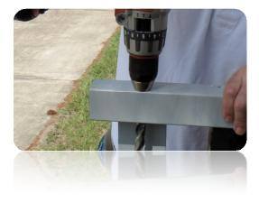
Drill a hole centered on the cross mark made using a 5/8" drill bit. Go completely through both walls of the frame.
