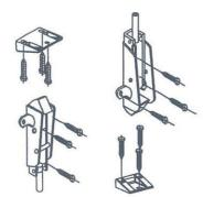
6) INSTALL TOP THREADED ROD INTO CONNECTOR PIECE ON TOP PULLMAN LATCH, HOLD THREADED ROD IN VERTICAL POSITION READY TO CONNECT WITH MAIN DEVICE.
